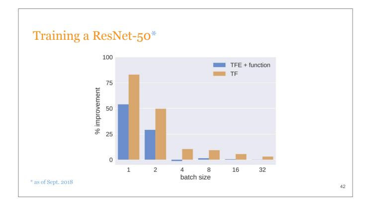
This slide is another way of looking at the Resnet-50 data. It shows the percent improvement in examples per second that TFE+function and plain TF have over TF. As the batch size increases, the improvement goes to zero ...
