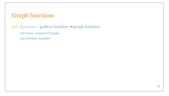
The @tf.function decorator is a just-in-time tracer. The first time the decorated function is run, it executes the Python function in a graph-construction context to generate an graph function. It is not a compiler for arbitrary Python functions.
