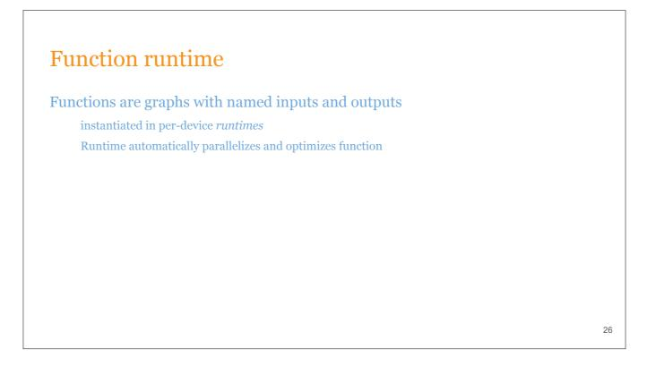
Functions are instantiated in per-device runtimes. The runtime automatically parallelizes and optimizes each function before running it. This is essentially the same execution model as classic, graph TensorFlow.
