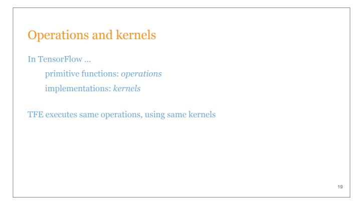
As a recap, in TensorFlow, primitive functions are called operations, and their implementations are called kernels.
