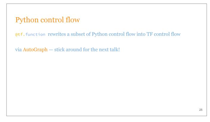
I lied, a little bit, when I said that tf.function was just a tracer. Even though @tf.function is not a compiler for arbitrary Python code, it can and does rewrite a subset of Python control flow into TF control flow. This is done via AutoGraph, which actually is the subject of the next talk. So make sure you stick around for that, it's a very cool technology.
