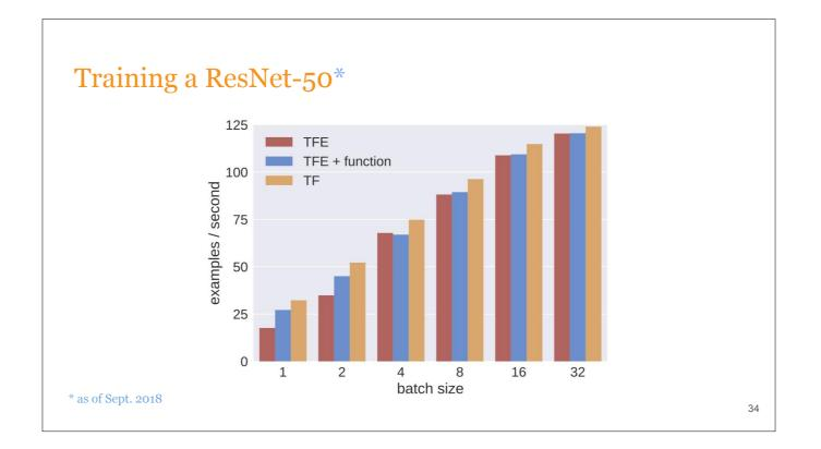
This chart shows the examples per second achieved when training a ResNet-50 on ImageNet on a GPU. The red bar is purely imperative TFE; the blue bar is TFE, accelerated by the function decorator; and the orange bar is pure TF.
